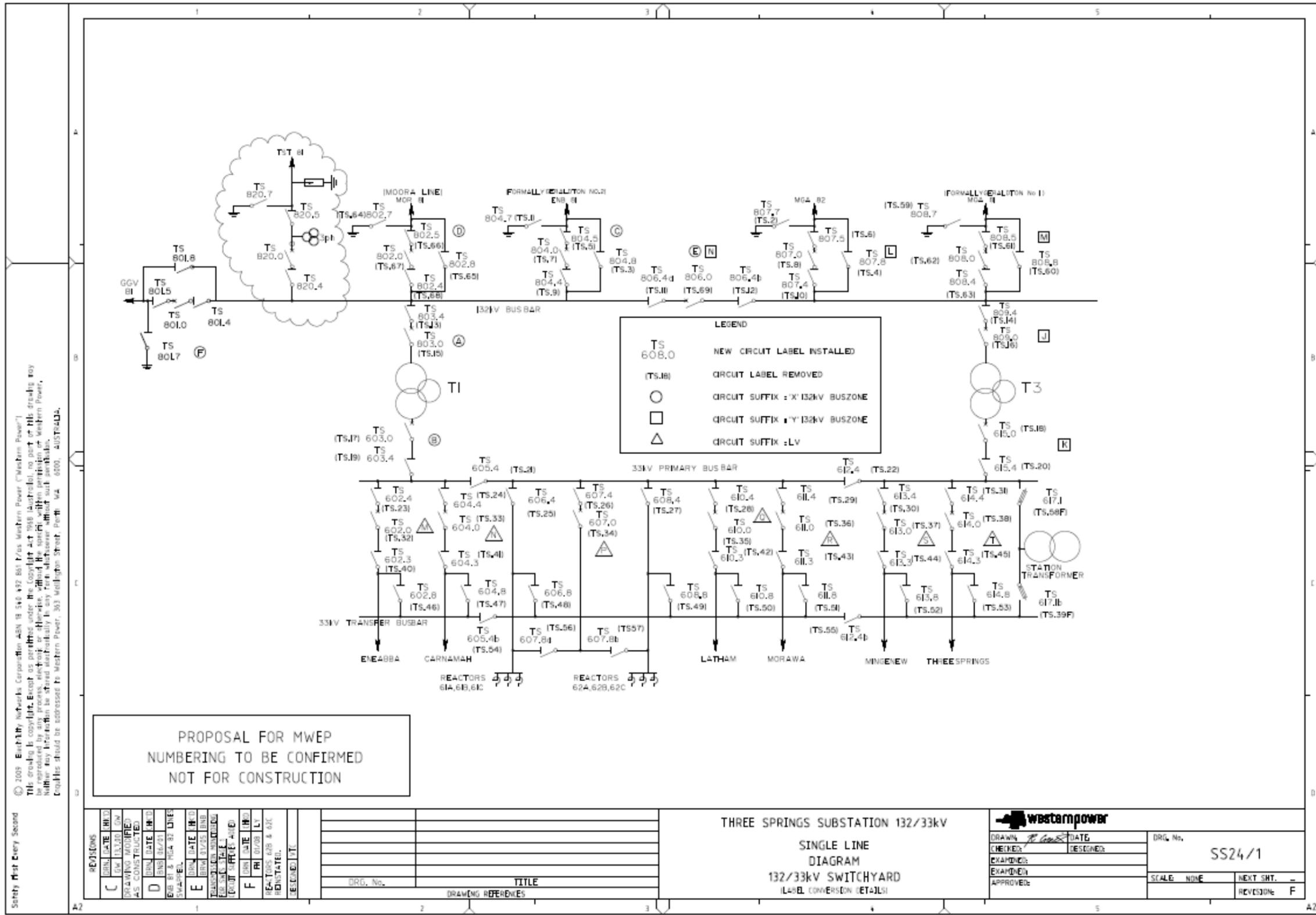
Figure D.3 TS 132/33 kV Single Line Diagram (showing new TST81 line)
