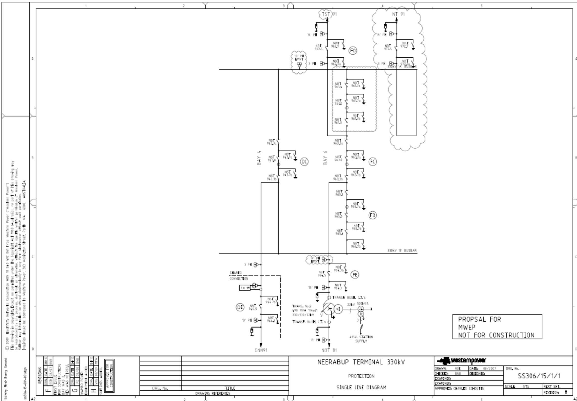
Figure D.1 NBT 330 kV Single Line Diagram (MWEP work shown clouded)
