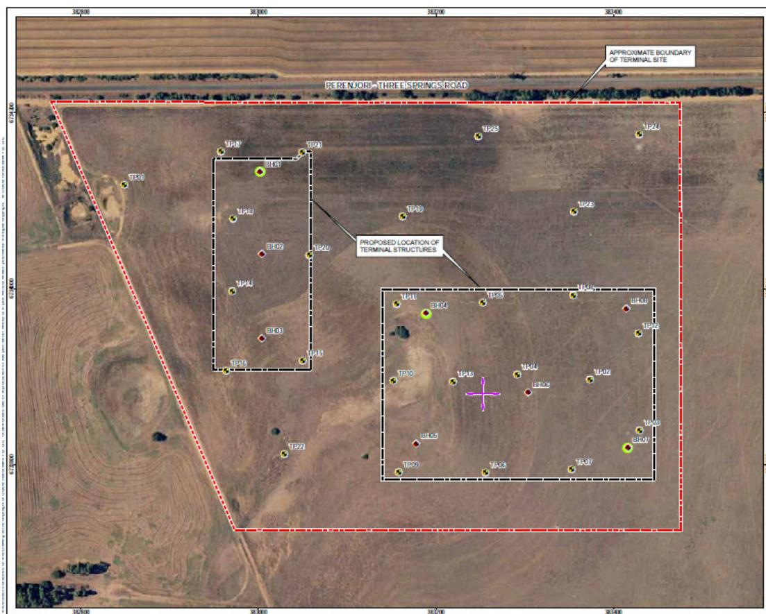
*Location of TST geo-technical test pits and bore holes*
